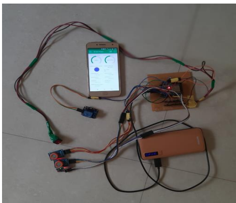
Fig 10: functioning of system when seat belt is not worn by driver and there is alcohol detection in car. So ignition relay is off. On dashboard android application we can see detection led glowing on app
