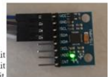
Accelerometer ,Gyroscope & surrounding Temperature Monitoring.
